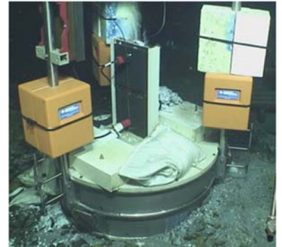
Hydrothermal Vent Power Generation Test Article, Deployed on Pacific Seabed
