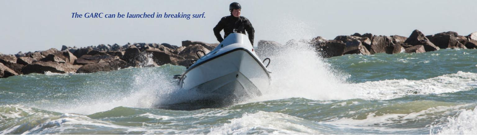
native to the high cost of outfitting disposable PWCs. That same year, Natick Soldier Systems Center certified the GARC for air drops from C-130s, something enabled in part by the Kevlar layer in the GARC's composite hull.
